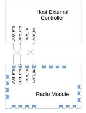
The serial UART communication needs to be configured with the correct parameters (baud rate, parity, start and stop bits) for successful communication.
